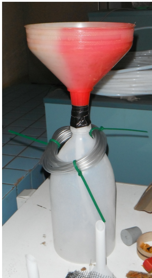
FIGURE 3.5: The rain event collector used in this study. The table tennis ball was placed at the top of the funnel inlet. The long tube twisted around the bottleneck is a pressure dumper. It allows the pressure equilibration between the ambient air and the bottle space avoiding any fractionation. The pluviometer was built following the IAEA guidelines for hydrological sampling.
