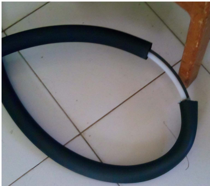
FIGURE 3.6: The sampling system setup used in this study consisted in a teflon tube (in white with o.d. 1/2 Inch), a self-regulating heating trace (in black) and a foam insulation (encapsulating both).
