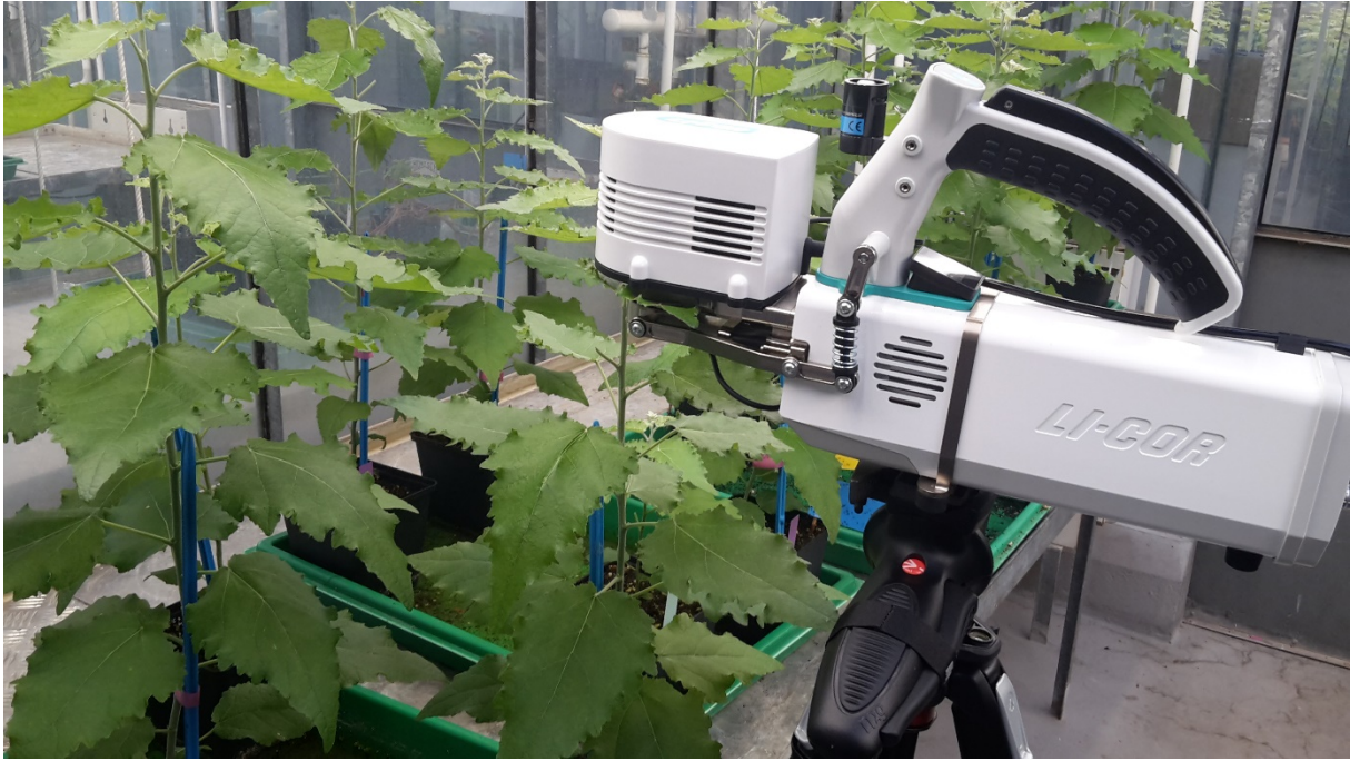
Figure 16: Photosynthesis measurement with the LI-6800 (LI-COR) system of a defined leaf from the top.
