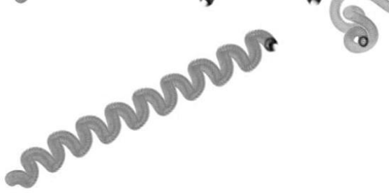
Figure 2.10 – Movie S5 showing one shell ( R_s \approx 30 \mu\text{m} , 131 s, speed x6 at 24 fps) ‘shark-fin’ meandering, with high persistence and periodicity, as well as a ‘curling’ single emulsion droplet, in a uniform bulk environment.
