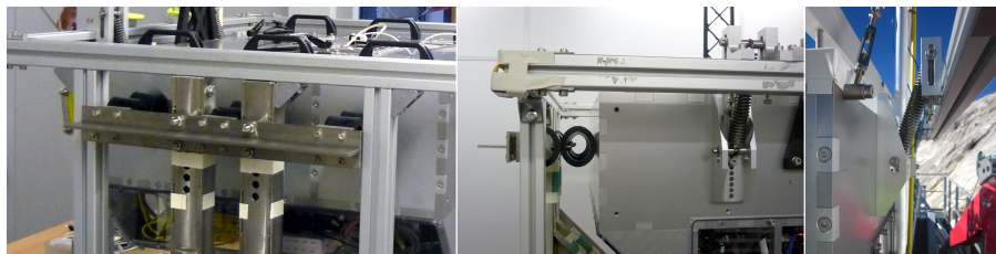
Figure 3.3: The camera box's suspension and buffers. Left: the buffers are adjusted, so when accelerating or decelerating, they push the box at the height of its centre of mass. Middle: overview of the springs and buffers; this viewing angle is comparable to the one in Fig. 3.1. Right: the camera box is suspended with extension springs. The springs are adjusted so that the camera box is level, and the spring attachment points are level with the box's centre of mass.
